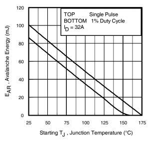
**Fig 16.** Maximum Avalanche Energy vs. Temperature
