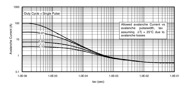
Fig 15. Typical Avalanche Current vs. Pulsewidth
