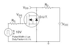
Fig 18a. Switching Time Test Circuit
