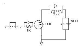
Fig 13b. Gate Charge Test Circuit www.irf.com
