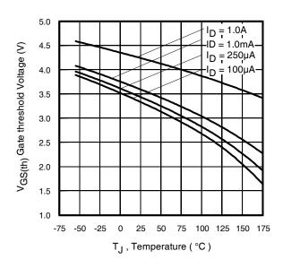
Fig 14. Threshold Voltage vs. Temperature
