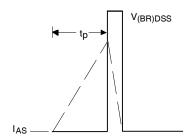
Fig 12b. Unclamped Inductive Waveforms
