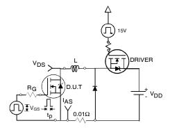
Fig 12a. Unclamped Inductive Test Circuit
