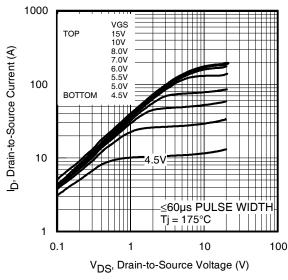
Fig 1. Typical Output Characteristics
