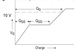
Fig 13a. Basic Gate Charge Waveform
