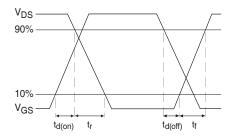
Fig 18b. Switching Time Waveforms
