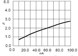
Relative Luminous Intensity vs Forward Current
