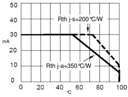
Maximum Forward DC Current vs Ambient Temperature
