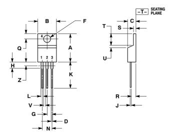
NOTES: 1. DIMENSIONING AND TOLERANCING PER ANSI Y14.5M, 1982. 2. CONTROLLING DIMENSION: INCH. 3. DIMENSION Z DEFINES A ZONE WHERE ALL BODY AND LEAD IRREGULARITIES ARE ALLOWED.
