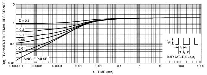
Figure 10. Thermal Response Junction-to-Case for MBR30H100CT
