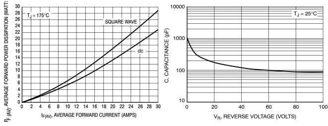
Figure 7. Forward Power Dissipation
