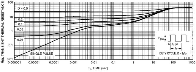
Figure 9. Thermal Response Junction-to-Ambient for MBR30H100CT
