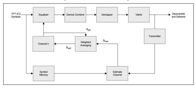
Figure 10: STBC Receive Block Diagram
