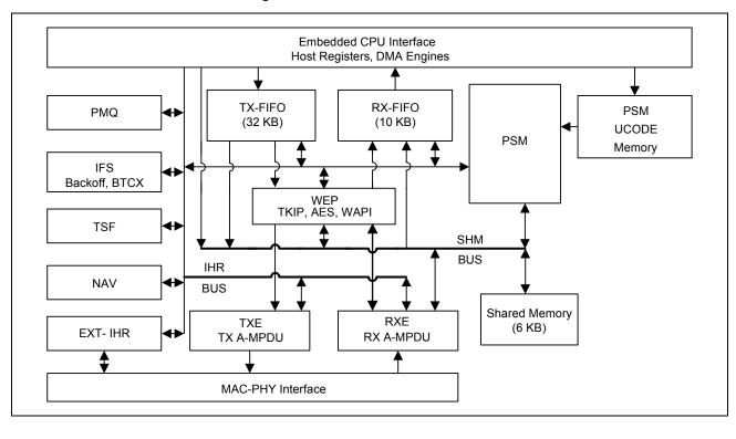
Figure 8: WLAN MAC Architecture
