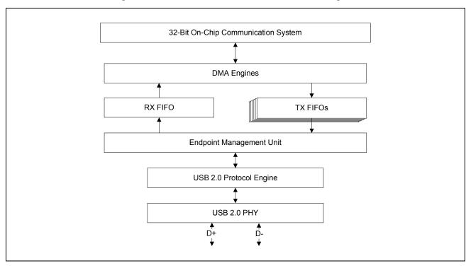
Figure 7: WLAN USB 2.0 Host Interface Block Diagram
