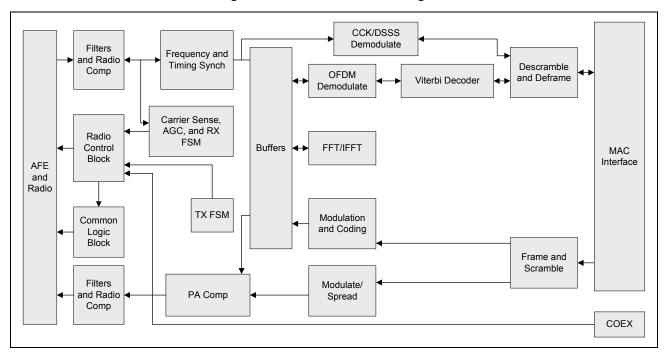
Figure 9: WLAN PHY Block Diagram
