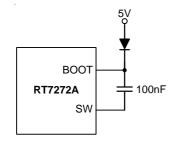
Figure 2. External Bootstrap Diode
