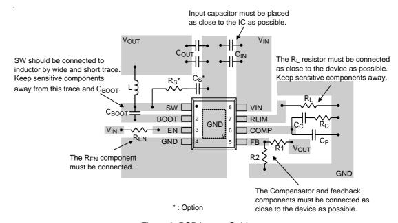
Figure 8. PCB Layout Guide
