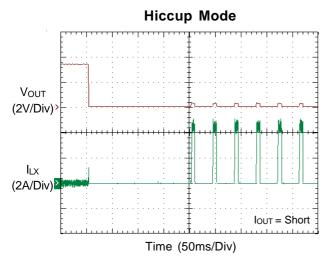
Figure 5. Hiccup Mode Under Voltage Protection
