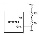
Figure 1. Output Voltage Setting
