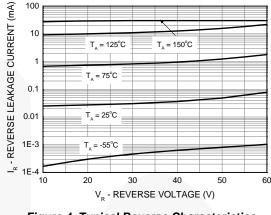
Figure 4. Typical Reverse Characteristics
