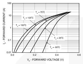
Figure 3. Typical Forward Characteristics
