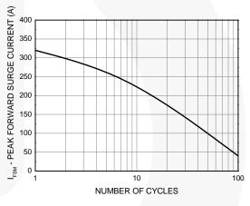
Figure 6. Maximum Non-Repetitive Peak Forward Surge Current
