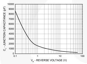
Figure 5. Typical Junction Capacitance
