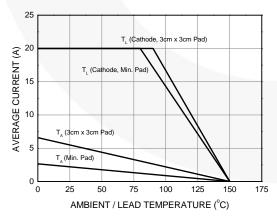
Figure 7. Forward Current Derating Curve
