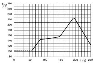
Fig.4 Maximum temperature load during infrared reflow soldering measured on the soldering pad
