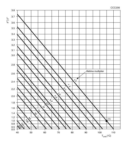
$I_A$  = actual ripple current at 100 Hz or 120 Hz  $I_R$  = rated ripple current at 100 Hz or 120 Hz at 105 °C For case codes 0405 to 1010 max.  $I_A/I_R$  = 2.4 <sup>(1)</sup> Useful life at 105 °C and  $I_B$  applied:
