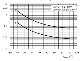
Fig.7 Typical dissipation factor (tan  $\delta$ ) at 100 Hz or 120 Hz as a function of ambient temperature
