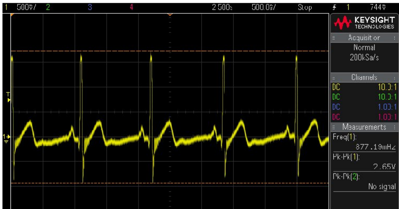
AFE module output when connected to a human subject in Lead II configuration using the modified Mason-Likar variant for electrode placement.
